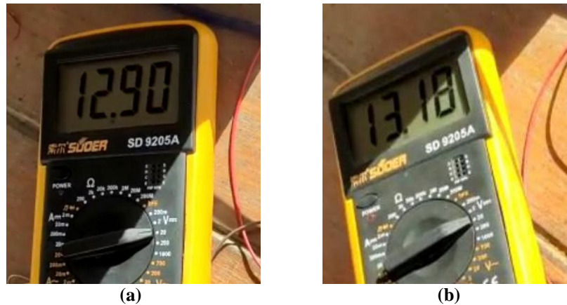
Figure 11: (a) battery before charging , and (b) after 5 minutes charging
